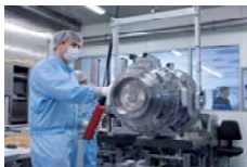
Assembly and alignment of a lithography optics system
