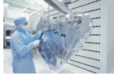
Assembly work on the illumination of the Starlith 3100, EUV optics from Carl Zeiss
