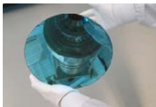
After several exposures, a silicon wafer like this turns into several microchips
