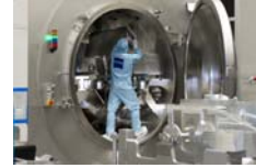
In the EUV cleanroom: employee working on a cleaning system for the illumination of EUV optics
