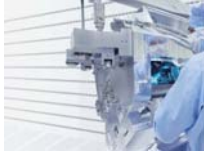
Assembly work on the illumination of the Starlith 3100, EUV optics from Carl Zeiss
