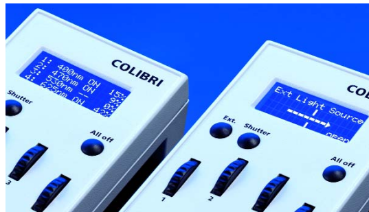
Control panel in LED mode with simultaneous use of three wavelengths (left) and after switching over to external white light source (right)
