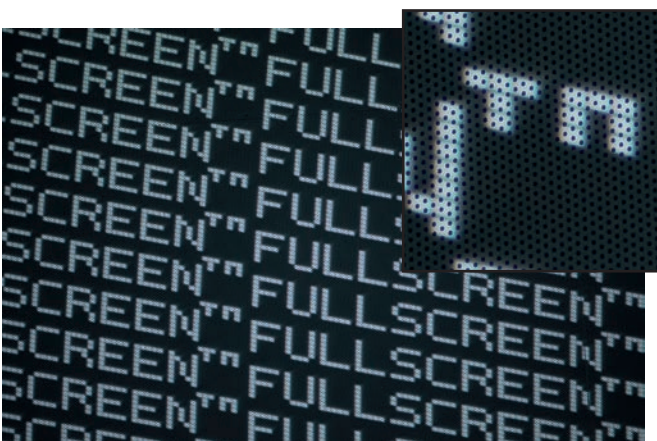
Segment of projected image, VELVET/DIGIGON 108 2.4/11.4 (test image) Lateral color: negligible – less than 1/4 pixel width; exposure data: Canon EOS 5D Mk II, ZEISS Macro-Planar 2/100, ISO 800, f/2, 0.4s.
