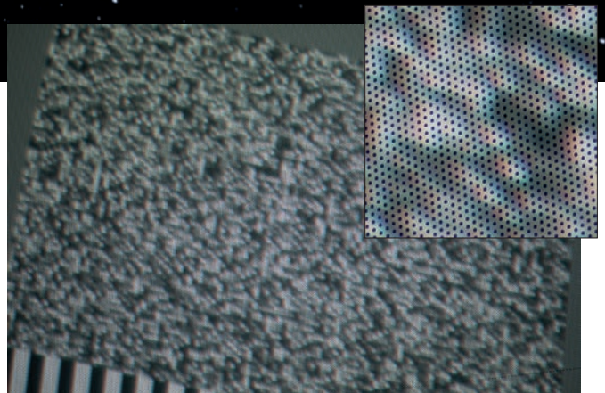
Segment of projected image, F35/NAVITAR HM117/11.7 – (test image) Definition: mediocre – pixels blurred; exposure data: Canon EOS 5D Mk II, ZEISS Macro-Planar 2/100, ISO 800, f/2, 1/8s.
